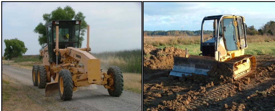
The Refuge System regularly uses heavy equipment such as road graders to maintain roads and bull dozers to create and maintain wildlife habitats such as wetlands.
